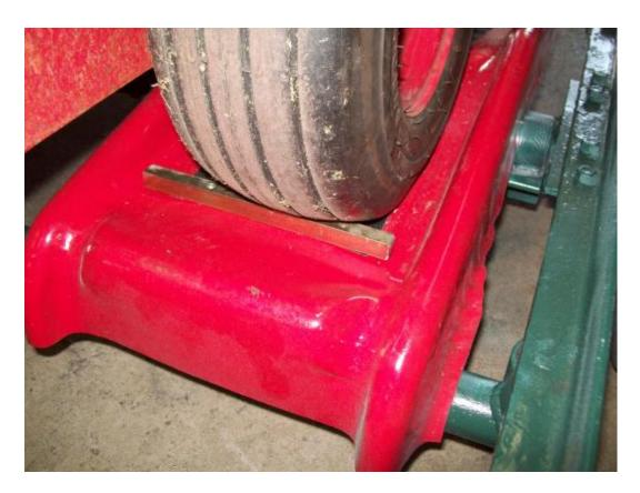
The tongue needed to be extended quite a bit so I added some pipe and then welded angle iron over the whole thing (2 sections so as to have a square tube. A standard tractor hitch is used to attach to the cart.
