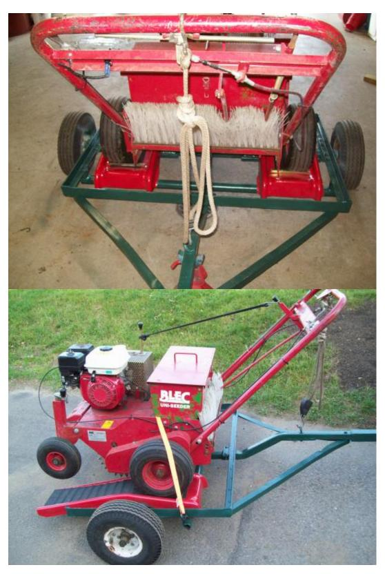
They can now load and off load the Blec without changing the front wheels which speeds things up a bit. We found that if the unit is in gear it controls the offloading when it is removed for storage as it tends to act as a brake.
