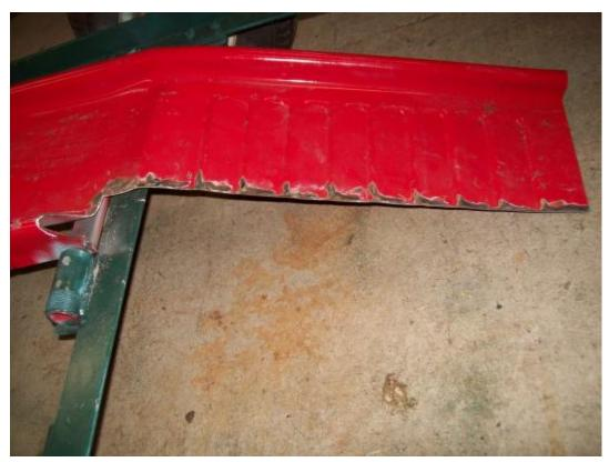
Next I cut the ramps to accommodate the spiker's and seed tubes, I also welded on a section of flat stock for support.
