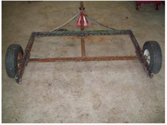
I cut the ramps down in height as it wasn't needed. To mount them I welded a section of pipe across them and fitted the pipe within another section of pipe so that they could pivot. The outer sections of pipe were welded to the trailer frame with and extra section of angle to mount them on.
